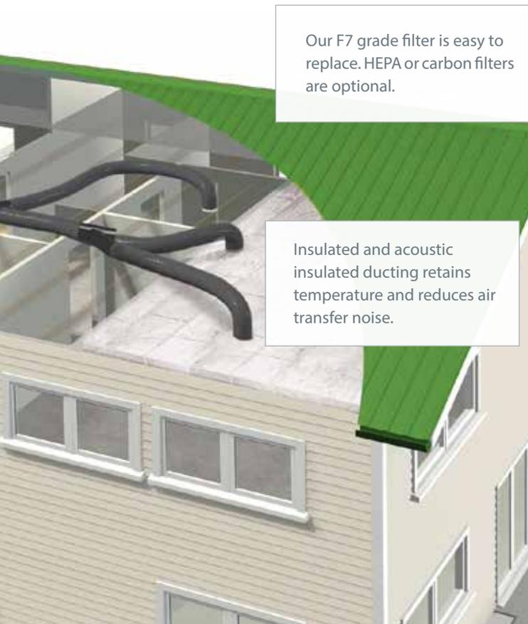
Our F7 grade filter is easy to replace. HEPA or carbon filters are optional.
