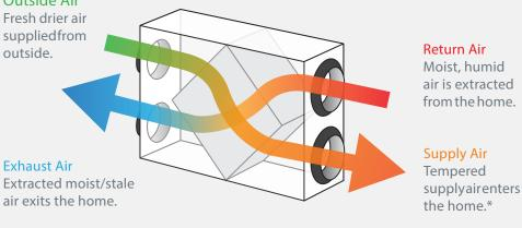
\*The temperature of the air supplied is influenced by the temperature inside and outside the home.
