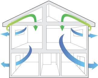
Outside Air Filtered drier air drawn from ceiling or outside. Exhaust Air Moist/stale air exits the home.
